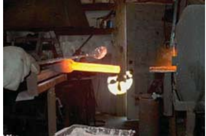
Fluxing the bar as it's being welded to an 160 layer pattern.
