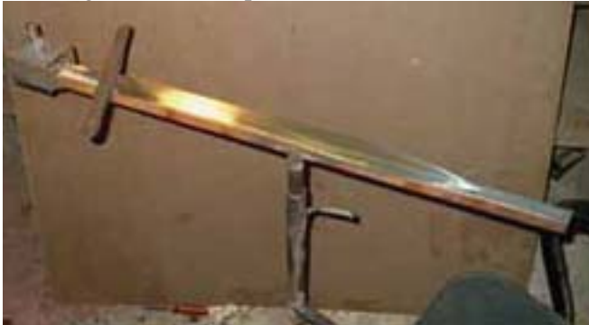
The blade is polished up to 600X (grit).
