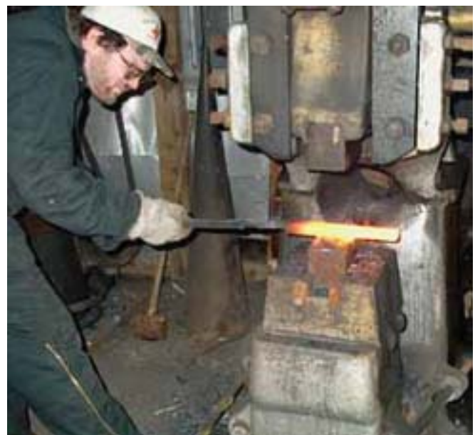
Drawing out the pattern welded bar that will eventually become the cross guard for the sword.
