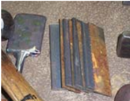
Billet peel (left) next to the alternating stack of mild steel and saw blades.
