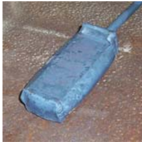
Completed billet removed from tube and stainless foil.
