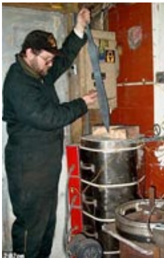
Figure 4 - Lowering the blade into the kiln point first to help reduce distortion.
