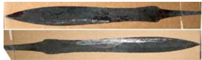
Figure 2 - Note the 'leaf' profile (the way the blade widens as it nears the tip). These changes in width affect grind angle which in turn necessitates leaving more material over all as a 'safety'.
