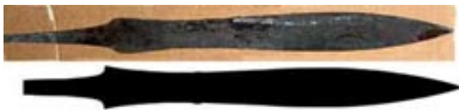
Figure 3 - Above is the final shape of the sword before grinding. Below is the template. Note the differences in the tang region that were necessary.
