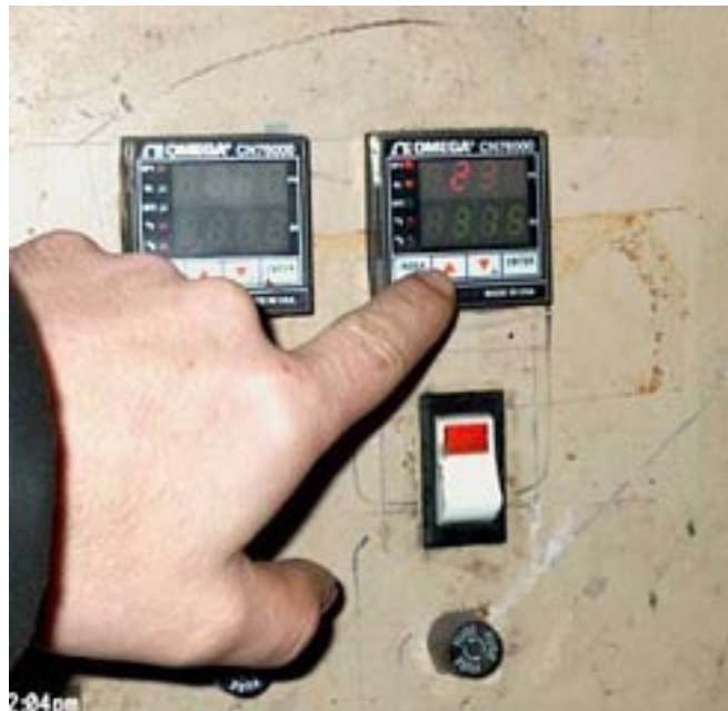
Figure 5 - Setting the controls on the kiln to 'soak' at 1375°F then cycle down to 900°F at -50°F/hr
